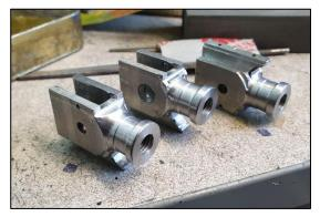
At this stage most of the machining has been completed, the stepped gudgeon pin holes have been cross drilled and counter sunk and the under cuts have been machined using the tool as mentioned above. After this picture there was a lot of hand work involved using a Dremel, files and sanding sponges.
