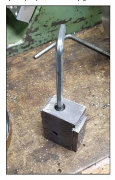
I have taken a different approach to make setting up a lot easier and less reliant on criticality. The piston rods are 5/16 stainless steel, I have threaded those 5/16 BSF and drilled/tapped the crossheads to match.
