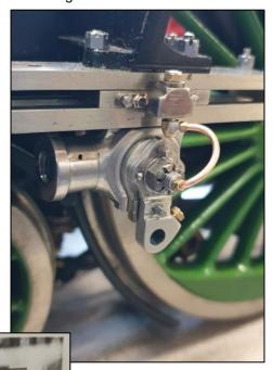
I have included this picture to show one of the reference photos used to get an idea of how the oil pipe sits. Note that we now have a true scale pipe, IIRC this is 0.5 mm OD and 0.3 mm ID. This pipe was tested using gear oil and timed for flow, it took 3 minutes for the oil to flow through the pipe when empty which for me seems good.
