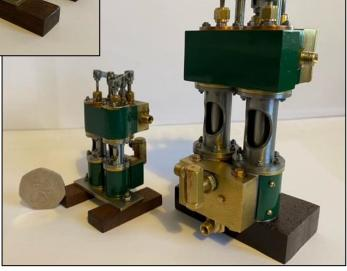
Consistent with the engines described last month no castings were used for either of these machines and it will be no surprise that both work very well.
