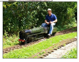
Being able to resurrect long gone locomotives has always been of great pleasure to model engineers. A shining example of this has been Gresley P2 three cylinder 2-8-2. After trial of the prototypes only four others of the type were built with the same wedge-shaped streamlining as the A4 pacific.
